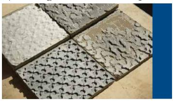
The significant residual mortar on both the tile and membrane after tiles are forcibly sheared demonstrates the outstanding strength.
